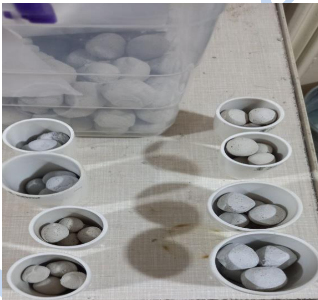
1-rasm. Laboratoriya sharoitida klinkerni tayyorlash bosqichi.
